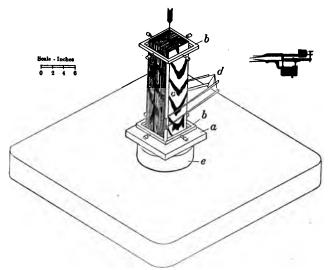
Fig. 5.—Compression parallel to grain.
